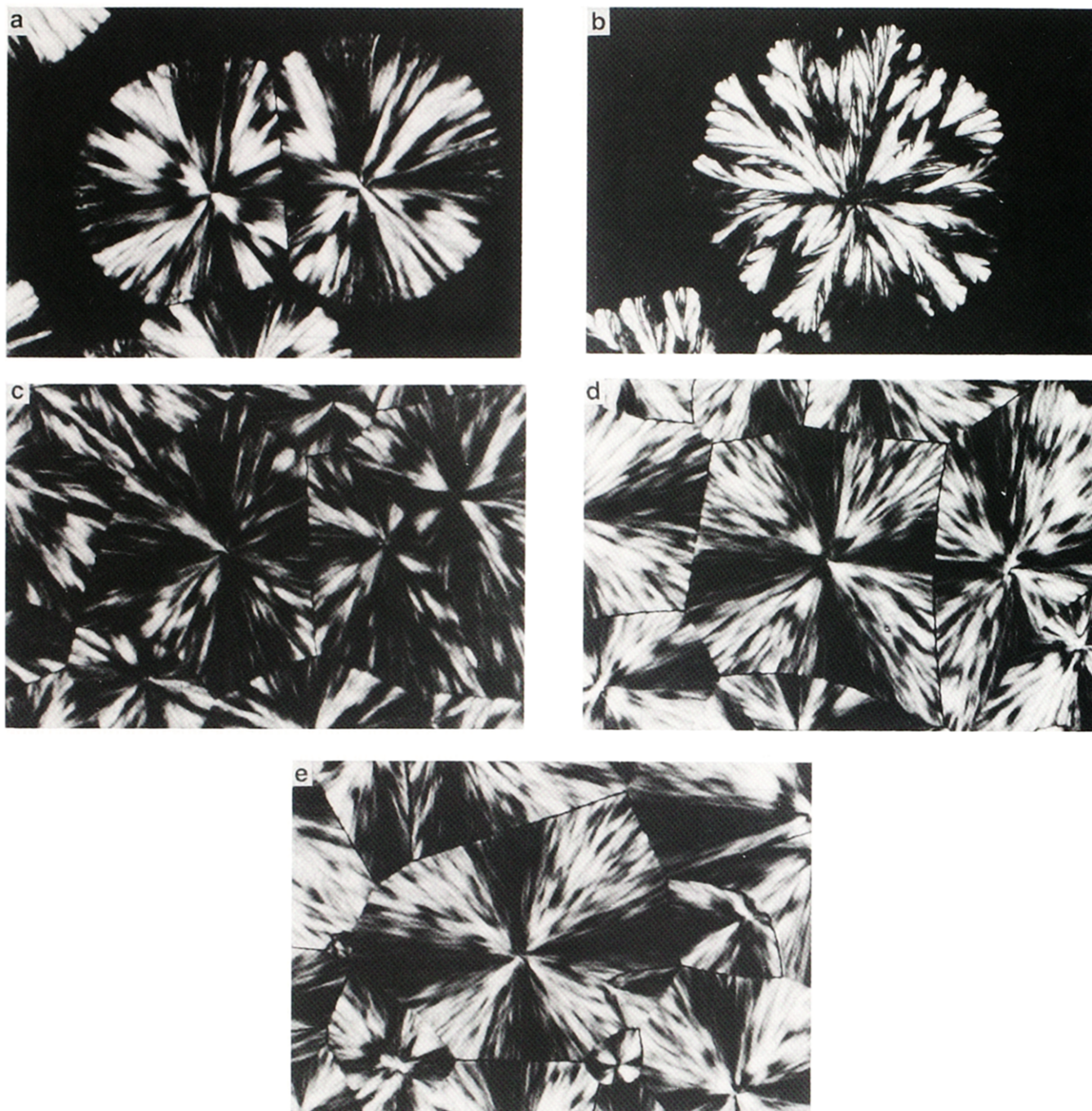
Figure 5 Polarized optical micrographs (1.8 cm = 30 μm) of spherulites crystallized at T_c = 150^\circ\text{C} for 38 h: (a) \delta = 713 \mu\text{m} ; (b) \delta = 134 \mu\text{m} ; (c) \delta = 28 \mu\text{m} ; (d) \delta = 5.9 \mu\text{m} ; (e) \delta = 0.38 \mu\text{m}
